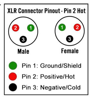
An easy way to remember the "Pin 2 Hot" wiring configuration, is to use the following trick:
